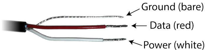
Figure 6: Pigtail End Wiring
