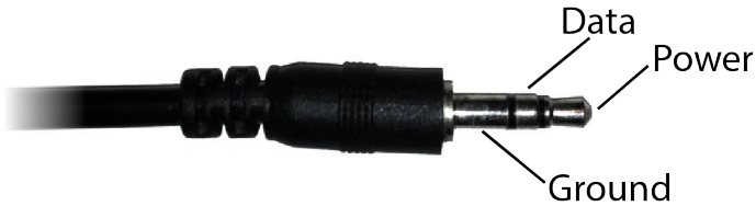
Figure 5: 3.5 mm Stereo Plug Wiring
